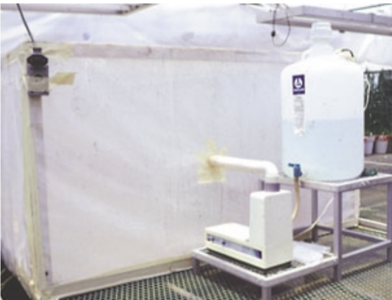
Figure 1.7. Ultrasonic humidifier modified to supply a cool mist of water in a plastic incubation chamber.
