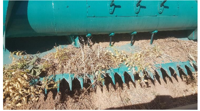
Fig.6- Soil in the combine's head due to short plant height and unlevelled land, rainfed chickpea field in Ghamlo, Kurdistan, July 25, 2019.
