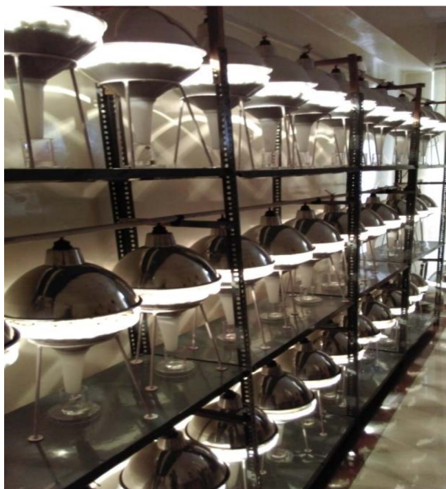
Fig. 1. Berlese-Tullgren funnels for micro-arthropods extraction. Each system contains a plastic funnel over which the wire mesh is placed and a collecting vessel below the funnel which contains a liquid preservative.
